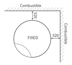
Clearances may be reduced with the application of heat shielding to walls in accordance to the Australian Building Code.
