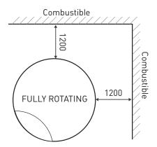
520mm minimum clearance is required if the rotation of the GyroFocus is locked at 120° or 90° away from the wall. Locking the GyroFocus so that the opening is fixed is an option available on purchase.
